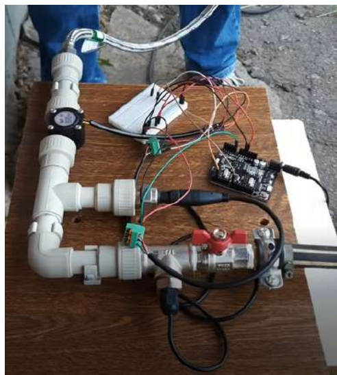
Fig.5. Full-scale model of the system of remote accounting and control of water consumption at production enterprises
