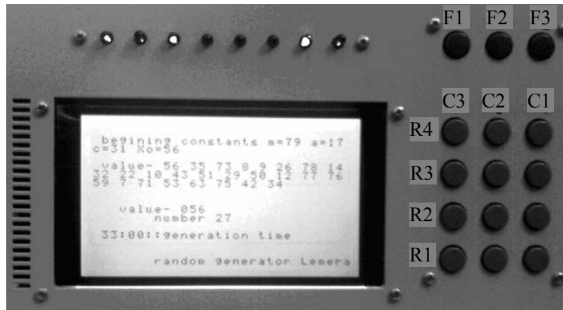
FIG. 1: Microcontroller-based (AVR-ATmega 128) laboratory breadboard construction
