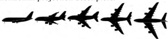
Figure 4 Change in the shape of the A380 aircraft's projection when the angle of the roll changes from 0° to 90°
