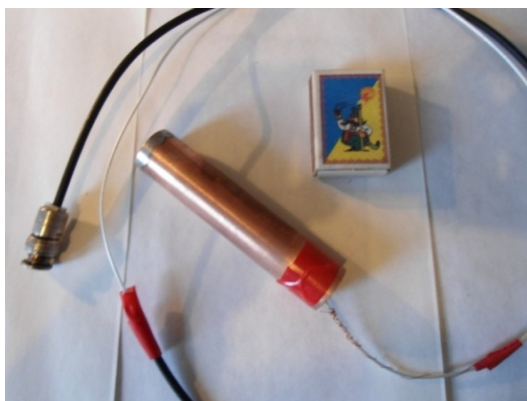
Fig. 3c. Appearance of a copper glass with established in it probes and connecting cable.
