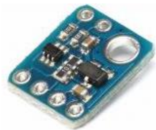
Fig. 7. Laser distance sensor GY-530 on VL53L0X.
