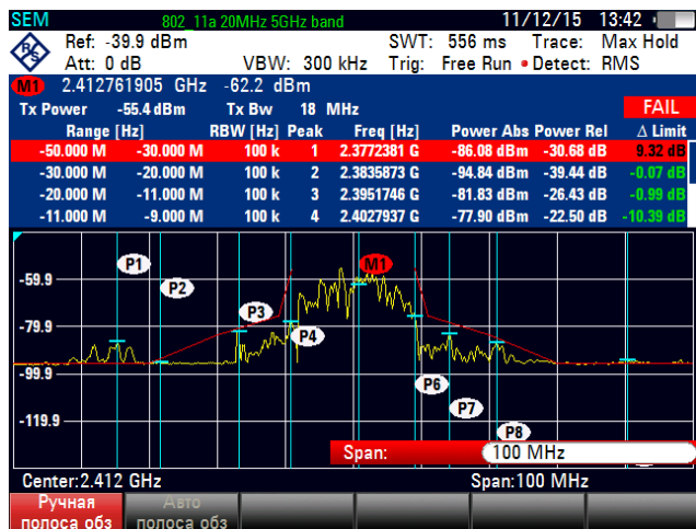
Fig. 2 - Screen View of the Rohde & Schwarz FSH-8 Spectrum Analyzer
