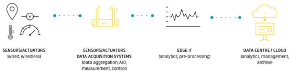
Figure 1.2. The four layers of IoT architecture described in detail
