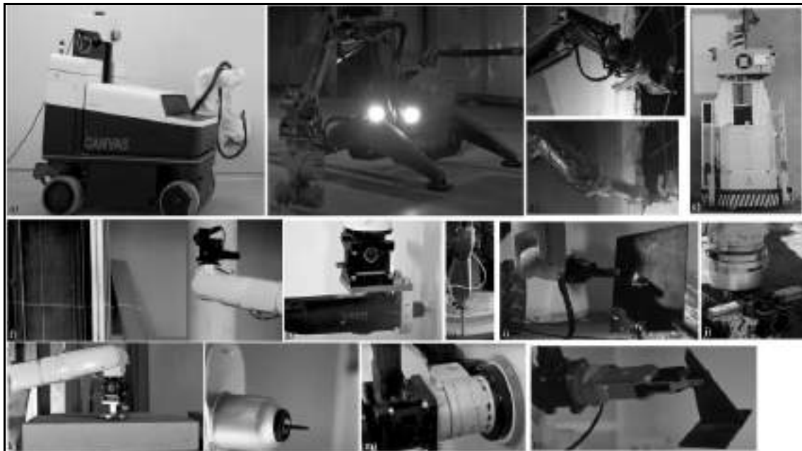
Figure 1 – Applications of manipulator-based construction robots a) – sanding; b) – crushing; c) – cutting; d) –jackhammering; e) – painting; f) – laser marking; g) – milling; h) – 3D-printing; i) – plasma cutting; j) – surface scanning; k) – ejectoral lifting; l) – screwing; m) – grinding; n) – object carrying [2][3]
