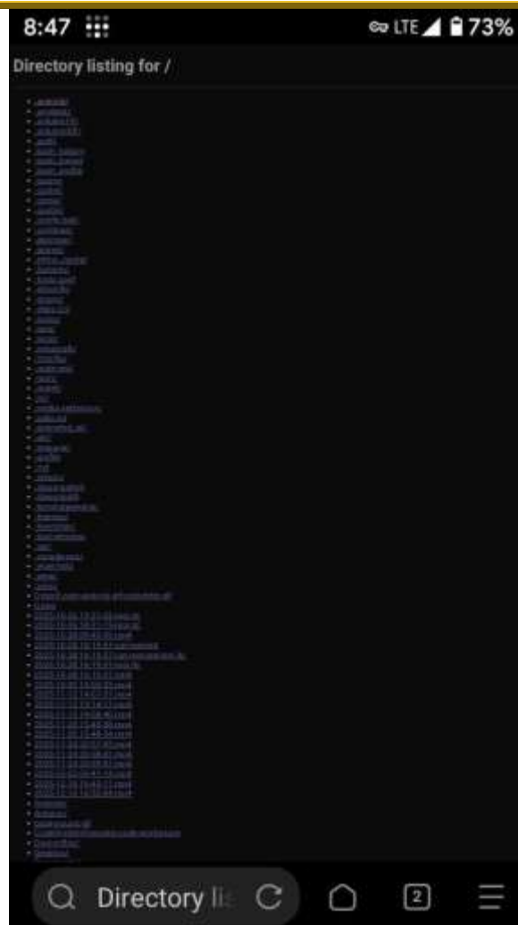
Fig. 7. Displaying the contents of the HTTP server directory of Node 1 in the browser of Node 2 through the Tailscale tunnel
