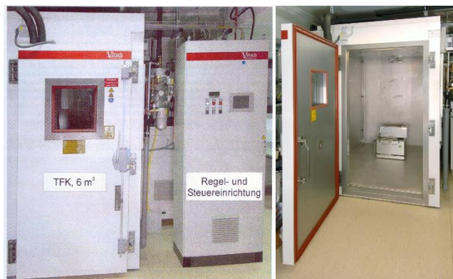
Fig. 2. Chamber of Thoron decay daughter products (PTB, Germany).
