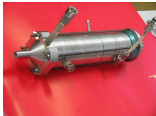
Fig. 8. Aluminum cassette implementing the "double filter" method.
