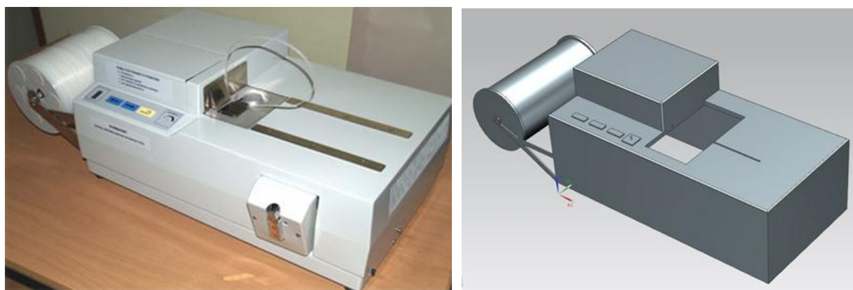
a) general view of the UNA 001 banknote packer; b) a 3D model of the UNA 001 banknote wrapper was developed
