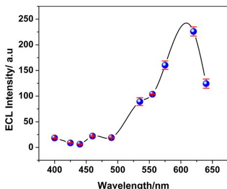
Fig. 2. ECL spectrum of RGL/Ru(bpy)<sub>3</sub><sup>2+</sup>. Conditions: 0.6 mM Ru(bpy)<sub>3</sub><sup>2+</sup> and 1 mM RGL in BR buffer (pH 7.2) on GC electrode; photomultiplier tube voltage: 1000 V.
