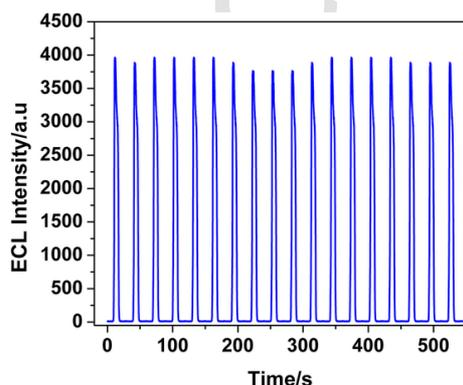
Fig. 4. ECL signal stability vs time; 0.6 mM  $\text{Ru}(\text{bpy})_3^{2+}$  and 1 mM RGL in BR buffer (pH 7.2) on GC electrode; Scan rate: 0.1  $\text{V s}^{-1}$ ; photomultiplier tube voltage: 1000 V.
