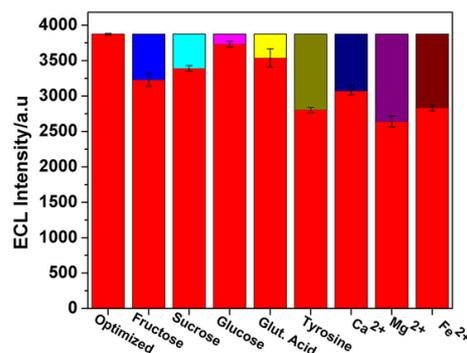
Fig. 5. Relative ECL intensity of the optimized RGL/ $\text{Ru}(\text{bpy})_3^{2+}$  system in the presence of the co-existing interfering species (IS). Conditions of the measurements: 0.6 mM  $\text{Ru}(\text{bpy})_3^{2+}$  and 1 mM RGL in BR buffer (pH 7.2) on GC electrode; concentration of the IS: 50  $\mu\text{M}$ ; scan rate: 0.1  $\text{V s}^{-1}$ ; photomultiplier tube voltage: 1000 V.
