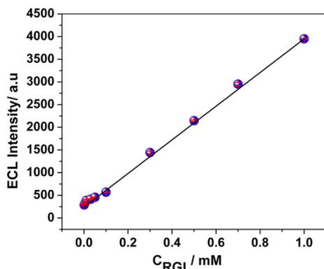
Fig. 6. The linear dependence of the ECL of the  $\text{Ru}(\text{bpy})_3^{2+}$  on the concentrations of RGL from 0.001 to 1 mM (1–1000  $\mu\text{M}$ ).  $c$   $[\text{Ru}(\text{bpy})_3^{2+}]$ , 0.6 mM; pH, 7.2; PMT, 1000 V.
