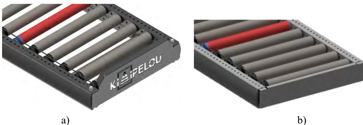
Fig. 8. General view of stop and start plates for roller conveyor: a) stop plate; b) starting plate
