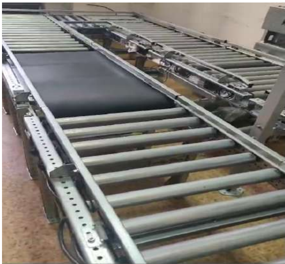
a) a fragment of an industrial roller conveyor with a belt zone
