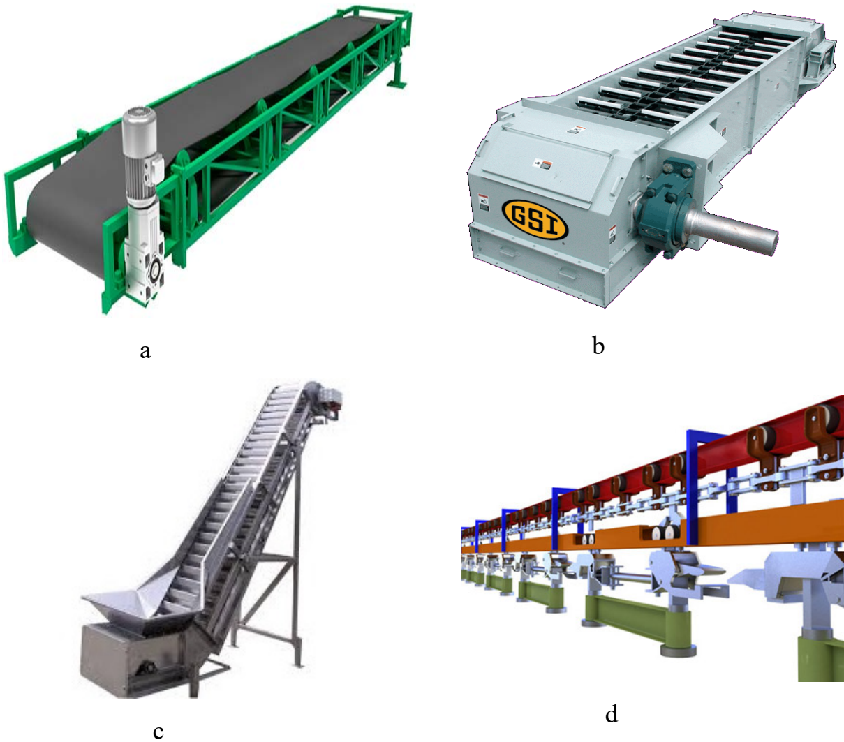
a – belt conveyor; b – scraper conveyor; c – bucket conveyor; d – overhead conveyor
