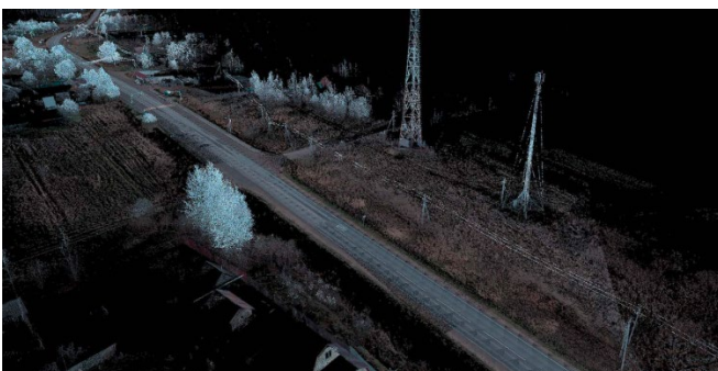
Fig.4. Examples of point clouds for road construction
