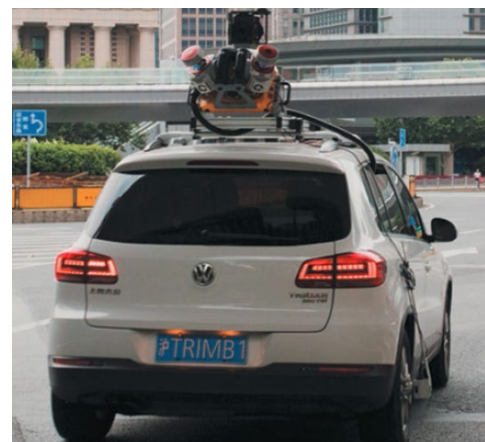
Fig.1. Scheme of Trimble MX 9 System and its vehicle mounting option
