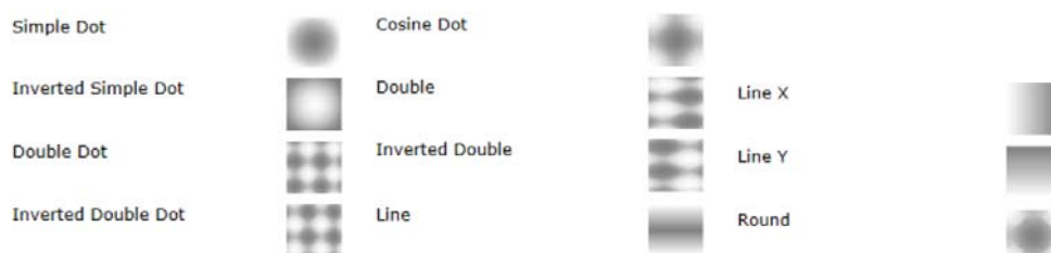
Fig. 1. Types of raster structures for Konica Minolta printing press
