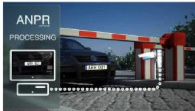
Figure 1 – Example of ANPR technology in operation [3]
