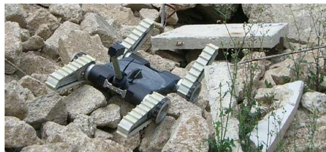
Figure 5. – Track robot rescuer analyzes the terrain[7]
