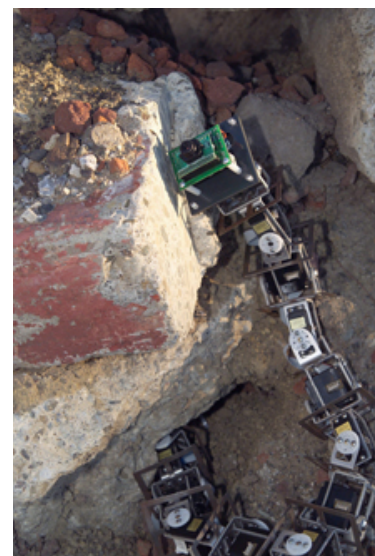
Figure 2. – The Snakebot as it maneuvers through the rocks. [4]
