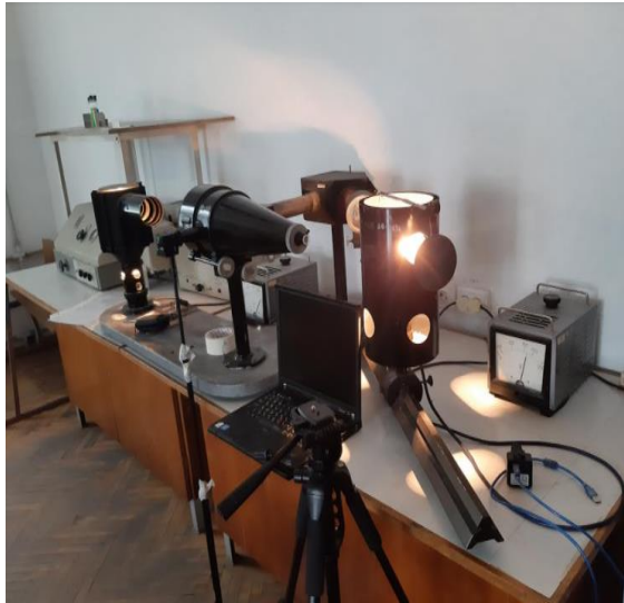
Figure 2 – General view of the installation of the camera spectrophotometer
