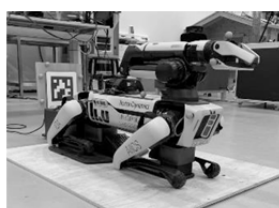
Figure 2 – Spot robot with AprilTag and reflective markers [11]
