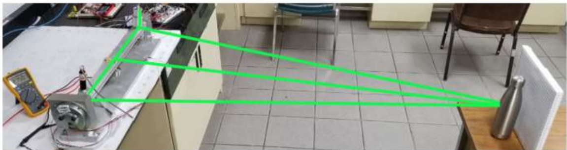
Figure 4.4 - Configuration of the positioning of the measurement object system in static triangulation
