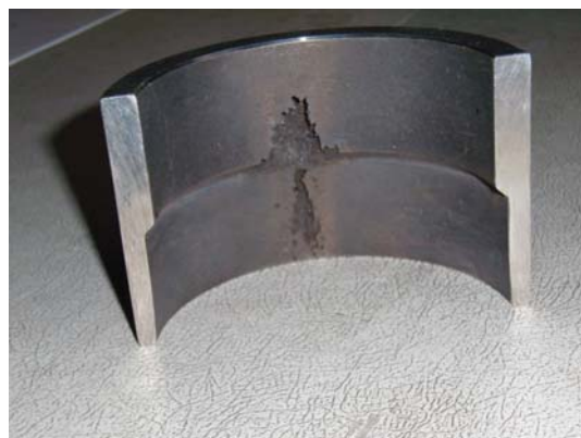
Fig. 1 – Fragment of the pipeline with a cavitation cave (defect).
