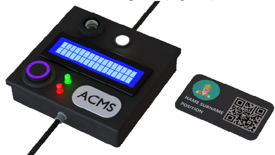
Figure 1. - Employee Identification System
