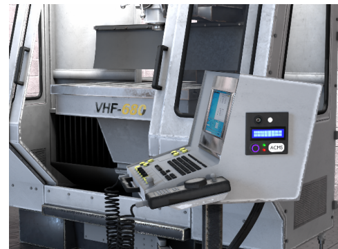
Figure 2. - Access Control System on the Equipment
