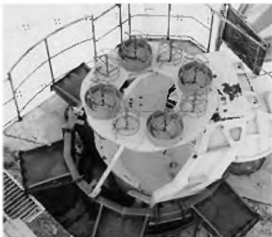
Figure 4. Feed system (327 MHz) and 6 feeds below with dual reflector frequency band selector (fig.2 shows one mirror of this beam-waveguide selector)
