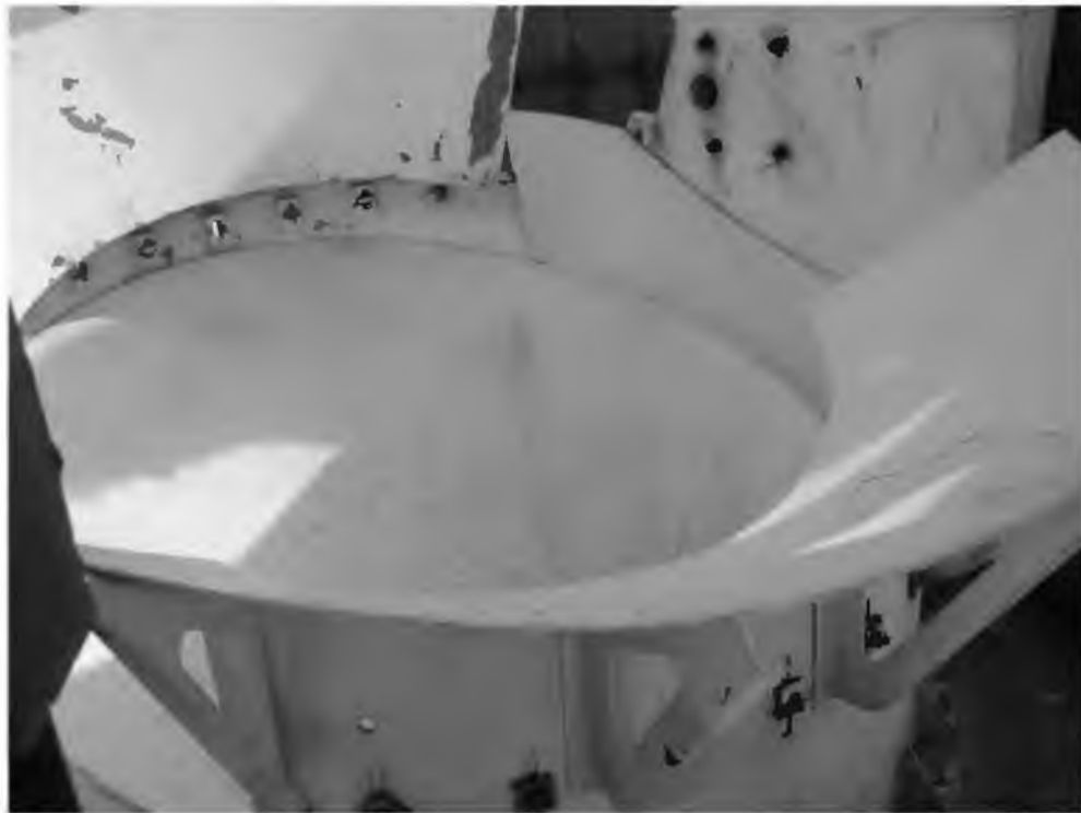
Figure 3. One of the reflectors in the dual-reflector band selector for frequency band selection, with diffracting edge elements, designed in the 80's [2]
