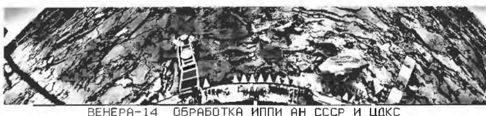
Figure 1. Panorama from Venera 14 Lander (Venus), low-gain antenna deployed at about 1/3 from the left
