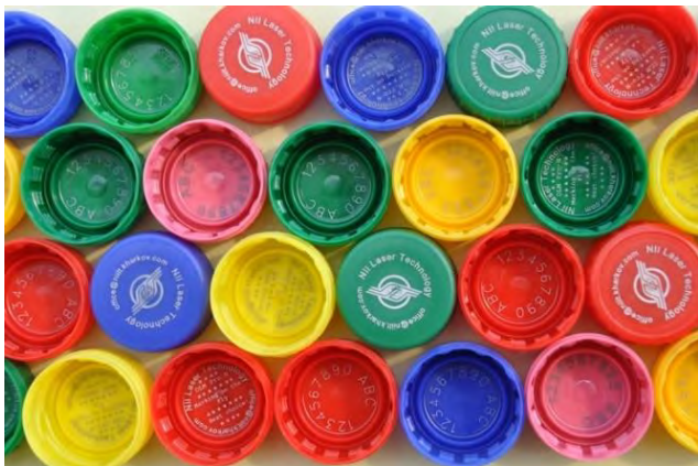
Fig. 4. UV laser marking on plastic closures.
