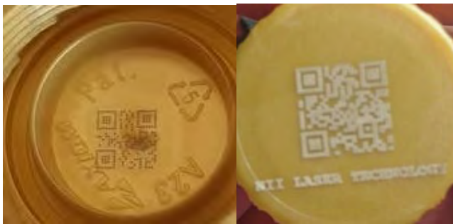
Fig. 6. An example of high-quality marking on bronze colored caps.
