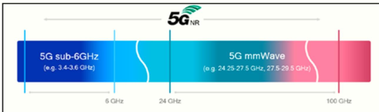
Fig.1. Extended spectrum for 5G NR (New Radio)
