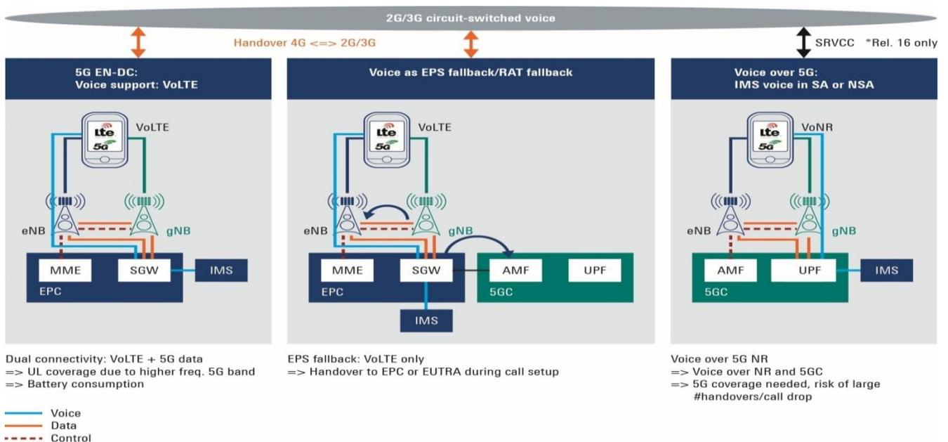
**Fig. 3. Existing mobile devices can use VoLTE or RAT fallback because native support for voice over 5G comes with 3GPP Release16**
