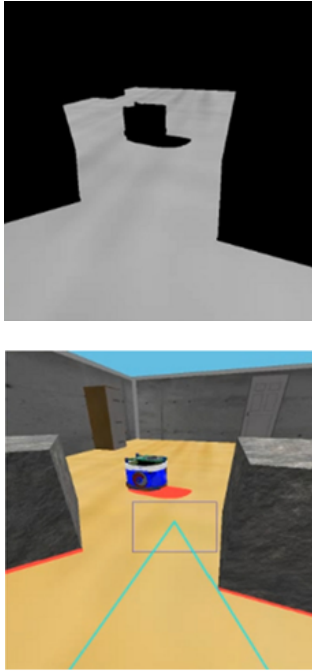
Fig.2 An example of video image processing using the navigation method based on the analysis of floor boundaries
