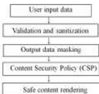
Fig. 1. Concept of protection against XSS attacks
