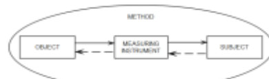
Fig. 3. Measuring instrument in the process of interaction between the object and the subject according to the measurement method
