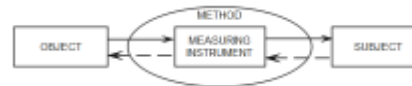
Fig. 4. Realization of the measurement method in the process with a complex measuring instrument (measuring system according VIM)
