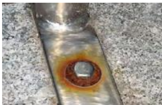
Figure 3 Standard case of contact corrosion
