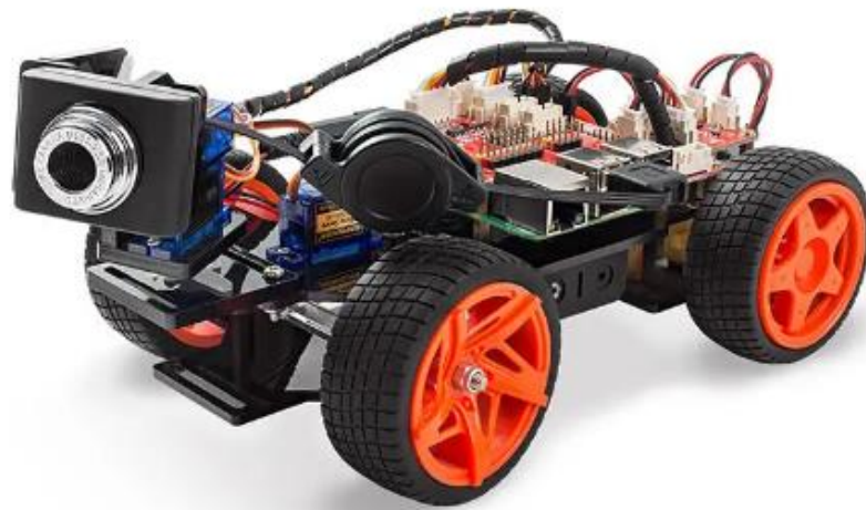
Рисунок 1.2 – Робот SunFounder PiCar-V Smart Robot Video Car V2.0 Kit for Raspberry Pi 3/2/B+ [7]
