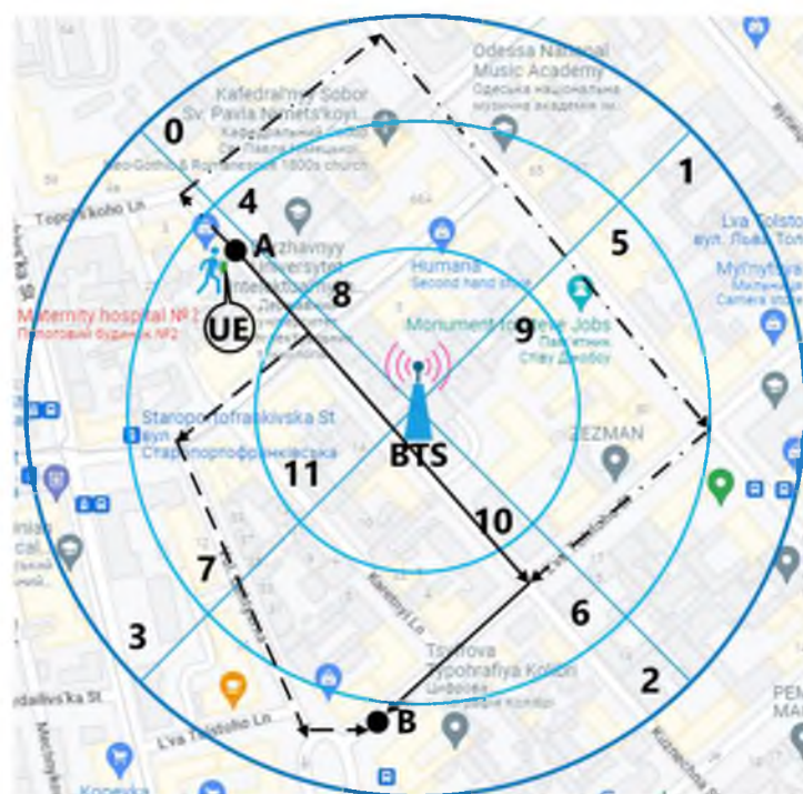
Fig. 4. Cell of a mobile communication system
