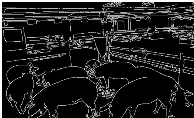
Fig. 6. The result of using the Canny detector
