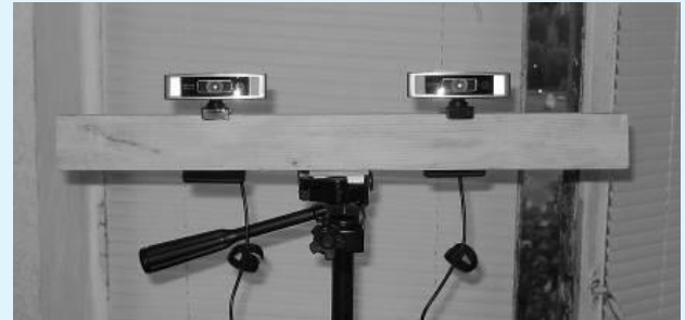
Figure 3a: Dual optical cameras used for surgical tool position determination.
