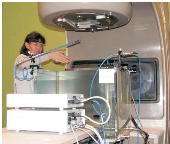
Fig.4. Experimental estimation of Varian Clinac 600C beam depth dose distribution in PTW water phantom
