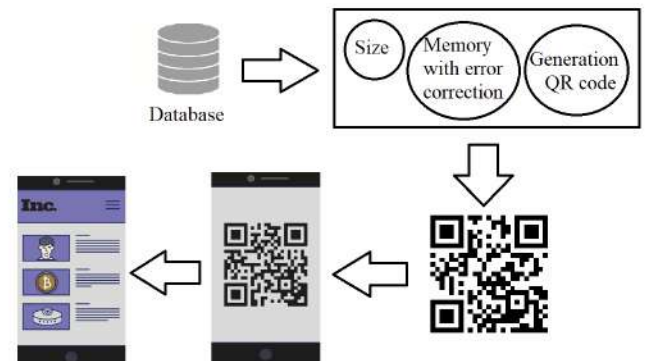
Fig. 2. Process of scanning QR code
