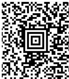
Fig. 5. Example of Aztec Code
