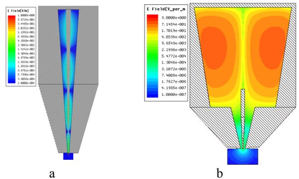
Figure 3 – Diagrams of the electric field for the RMC with different accumulative area: a) conical coax; b) volumetric RMC with a coaxial output
