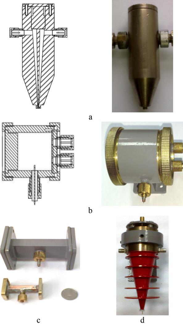
Figure 2 – RMC constructions: a) conical coax; b) a cylindrical; c) based on the waveguide segments; d) conical coax with the hybrid structure of the field
