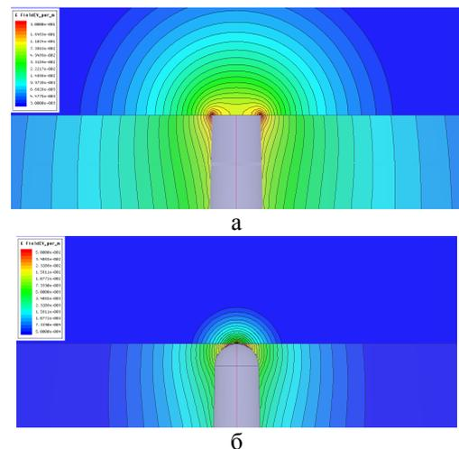
Figure 4 – Diagrams of the electric field in the aperture of the conical coaxial RMC with different tip shape: a) flat; b) spherical
