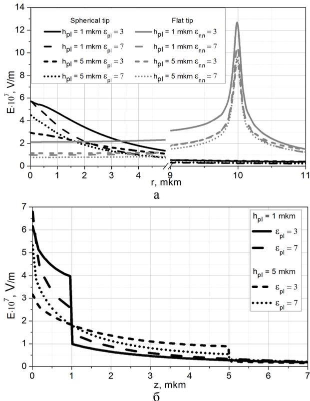
Figure 5 – The distribution of the microwave electric field along the surface (a) and the depth of the object (б)
