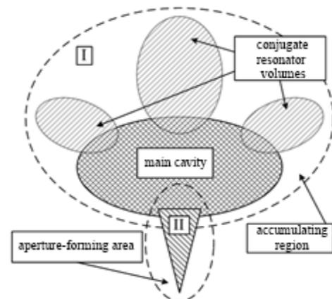
Figure 1 – A generalized schematic illustration of RMC
