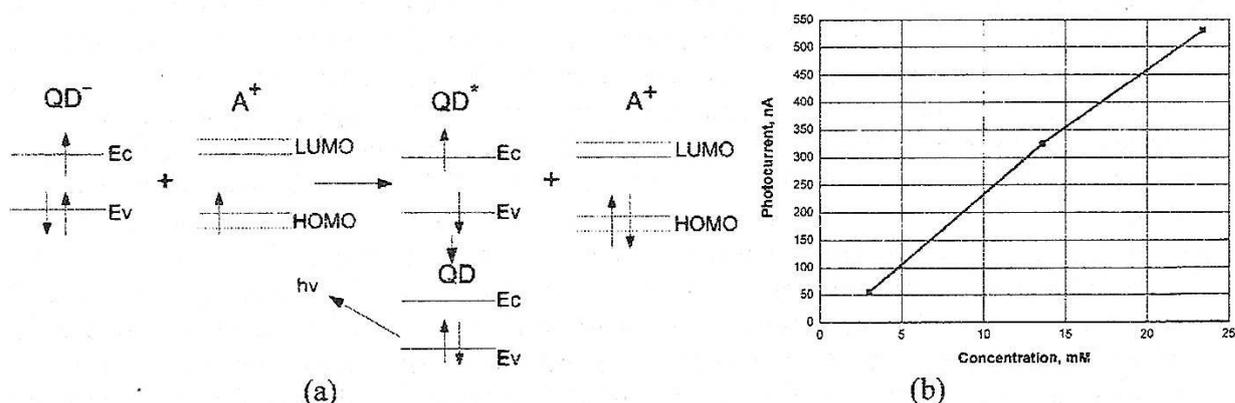
Fig. 1. Scheme of the process for polycyclic aromatic hydrocarbons detection: Ec – QD's conduction band; Ev – QD's valence band; LUMO – lowest unoccupied molecular orbital, HOMO – highest occupied molecular orbital (a); concentration dependence of photocurrent of the model tryptophan solution (b).
