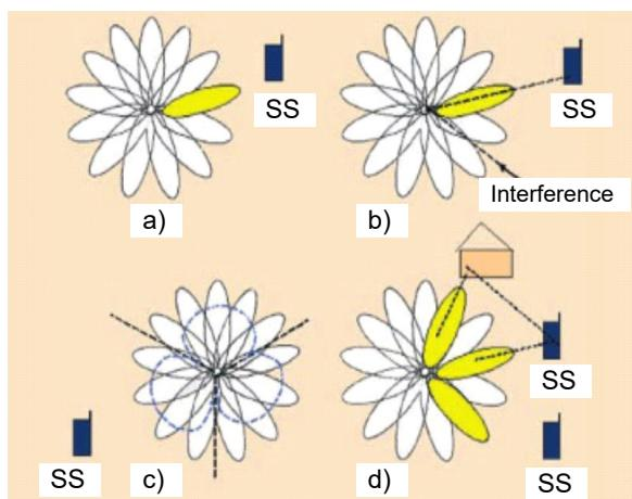
Fig. 1. Options of organization of multi-beam antenna
