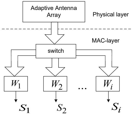
Fig. 2. The scheme SDMA of finding VWC individual assessment values of the base station
