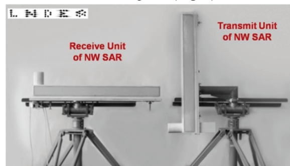
Fig. 2: Ground Based Noise Waveform SAR for MIMO mode with time division of Tx and Rx channels
