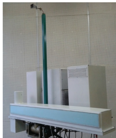
Fig. 5. Ground Based Noise Waveform SAR with horn transmit antenna
