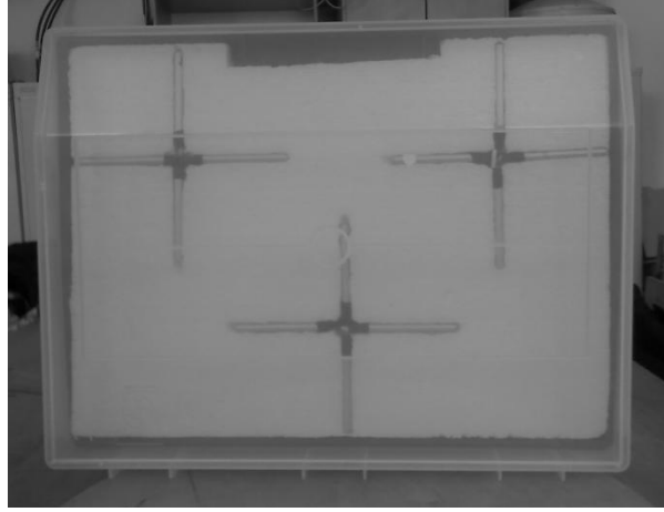
Fig. 3 – Real experimental polarization antenna for MIMO
